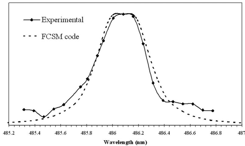
**FIGURE 3** Experimental  $H_\beta$  spectral line (solid line) and the simulated profile by FCSM model (dots) at  $T_e = 2.5 \text{ eV}$  and  $N_e = 3.16 \times 10^{21} \text{ m}^{-3}$ .
