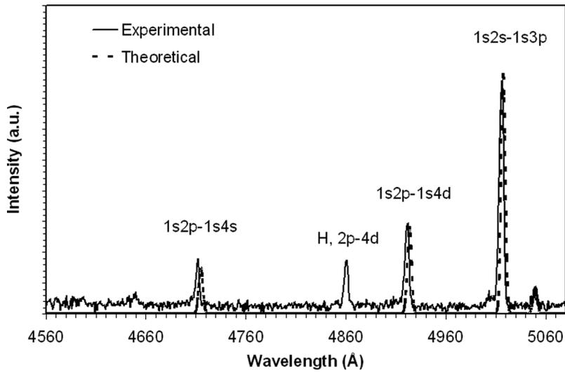
**FIGURE 2** Experimental He I spectral lines (solid line) and simulated spectrum by CRM (dots) for a  $T_e = 2.5 \text{ eV}$  and  $N_e = 3.1 \times 10^{21} \text{ m}^{-3}$  at a pressure of 0.3 torr.
