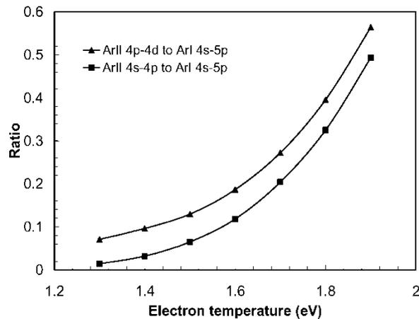
**Figure 4.** Line ratios of Ar(II) 4p-4d to Ar(I) 4s-5p line and Ar(II) 4s-4p to Ar(I) 4s-5p as a function of electron temperature in eV.
