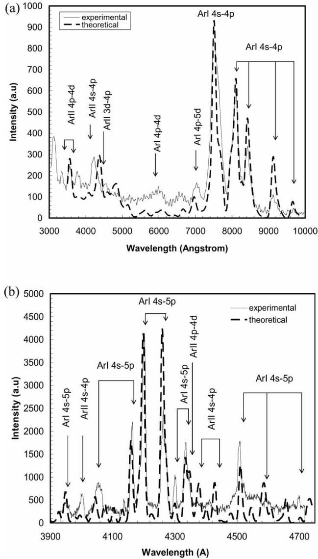
**Figure 2.** The experimental Ar(I) and Ar(II) spectrum from the glow discharge plasma superimposed on the theoretical spectrum: (a) spectrum between 300 nm and 1000 nm, (b) spectrum between 390 nm and 470 nm.
